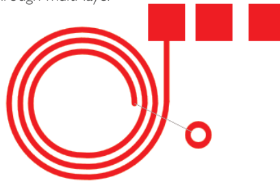
Define spirals for planar transformers spanning multiple layers
